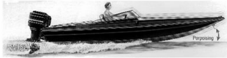
Figure 7-20 Engine or drive trimmed 'out' (bow too high). Porpoising
