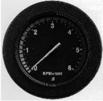
Figure 7-29 A tachometer measures engine revolutions per minute (RMP).
