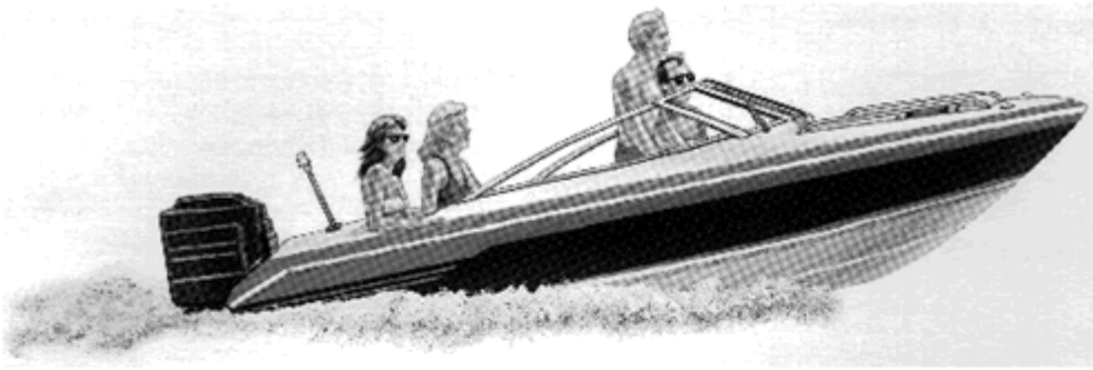
Figure 7-34 Weight concentration far aft is often preferable for top speed but still has some disadvantages.
