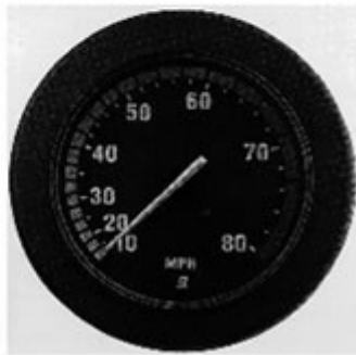
Figure 7-30 A speedometer measures boat speed in miles or kilometers per hour or knots
