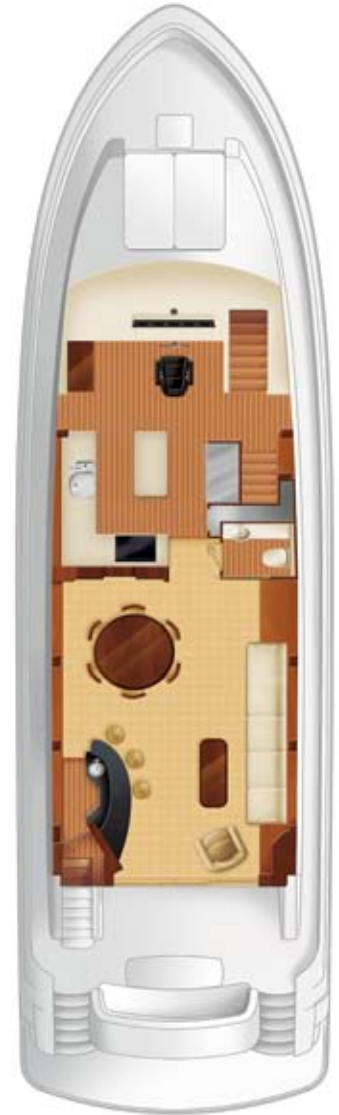
Optional Upper Deck Arrangement with Sunken Bar Lower Helm and Day Head
