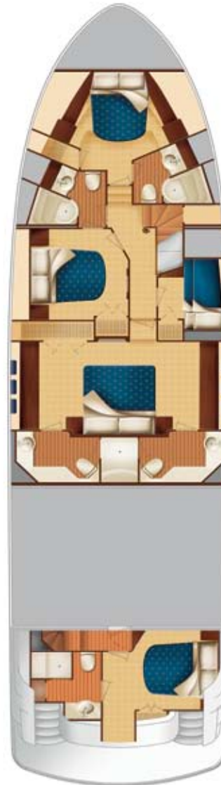
Optional Lower Deck with Four-Stateroom / Three-Head Arrangement, Aft VIP, and His & Hers Head in Master
