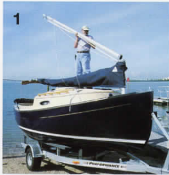
1 & 2 Untie and lift the mast to vertical.
