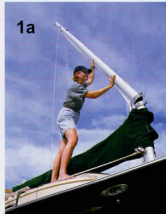
1a Untie and lift the mast to vertical. It's really very light.
