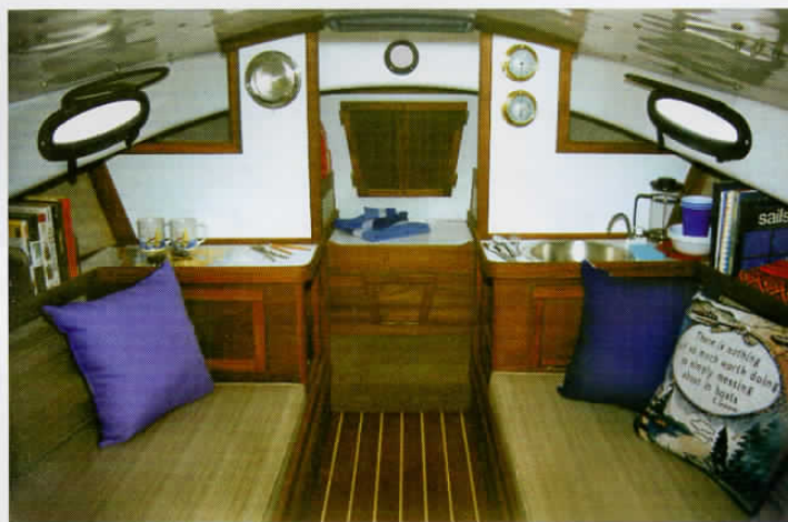
Because the centerboard trunk is completely enclosed beneath the sole, the Horizon Cat's interior is remarkably expansive and completely unobstructed.
