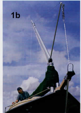
1b Place mast strut on mast. Winch mast to vertical using the forestay extension line.
